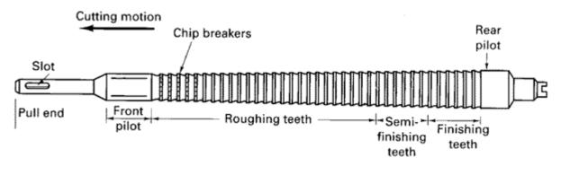
Figure 3. Parts of a broaching tool.
