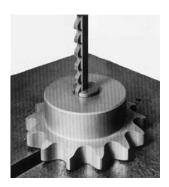
**Broaching with One-Pass Keyway Broaches** No shims are necessary. "C" style bushings are required. **1.** Insert bushing in part.
