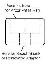
Ram Adapter to guide broach shank: When using special broaches, all D, Double-D, and most rectangular broaches have a tendency to deflect. To prevent this, the simple ram adapter, which can be fitted to either an arbor or hydraulic press, will guide the broach throughout the cut.
